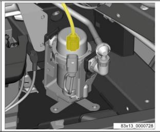
Make pass the connector through the rubber cover and install it onto the pump.
